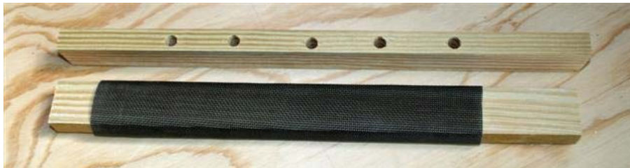
Lower vent to place between 1" x 4" corner pieces on bottom sides of tower
